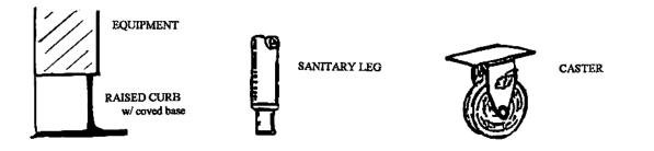
All stationary equipment must be sealed to the walls or be moved away from the walls at least six inches for every four linear feet of equipment length. Equipment must be spaced at least six inches apart from each other or be sealed together.
