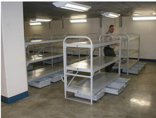
These triple bunks not only create an extremely close housing environment, they limit the visibility of inmate areas by staff when they are occupied. It should also be noted that upon examination, these bunks were not “correctional grade” fixtures that do not allow tampering.
