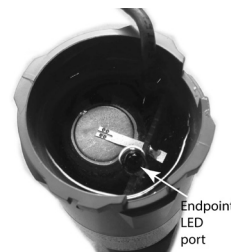
Figure 15: IR LED port ORION ME endpoint (bottom up view)
