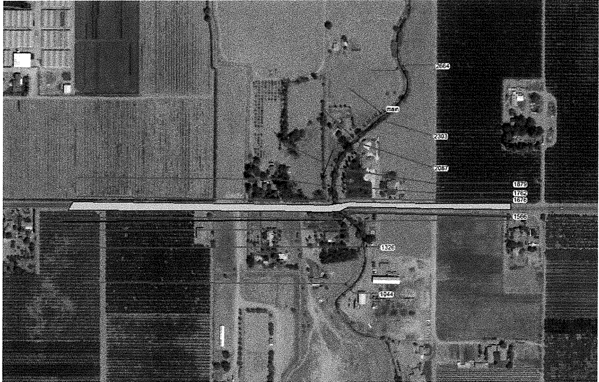
Figure 1: Plan view of HEC-RAS cross section
