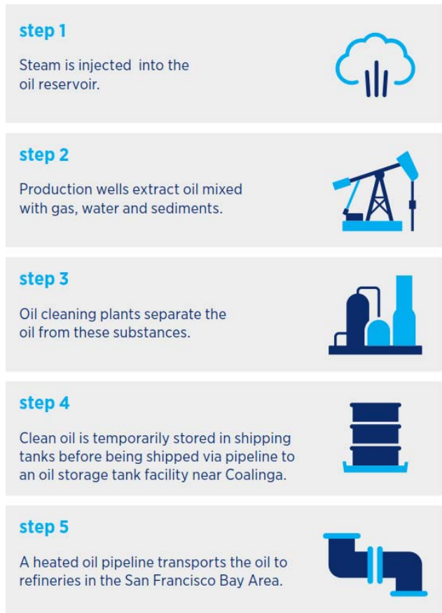
Figure 2-Typical Operations Oil Steam Extraction
