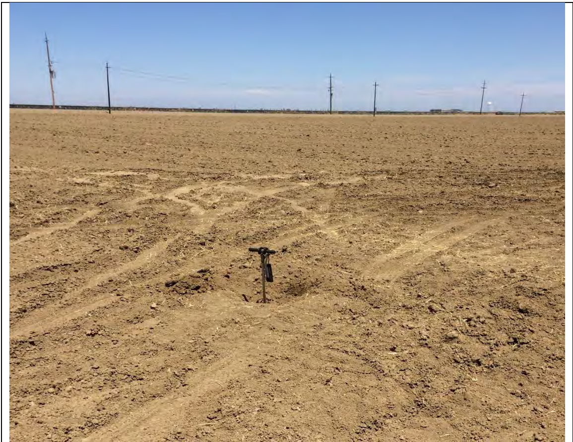
LPR driven into soil at TP-1
