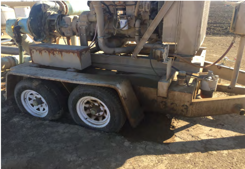
Site 5: Soil staining on and below trailer.
