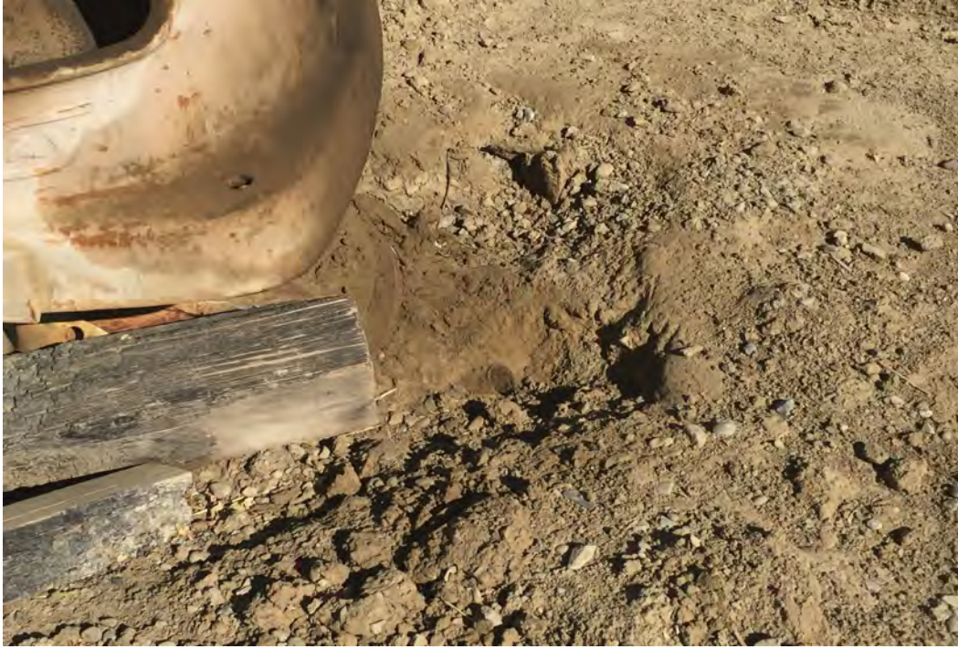
Site 3: Soil staining around base of ag pump.
