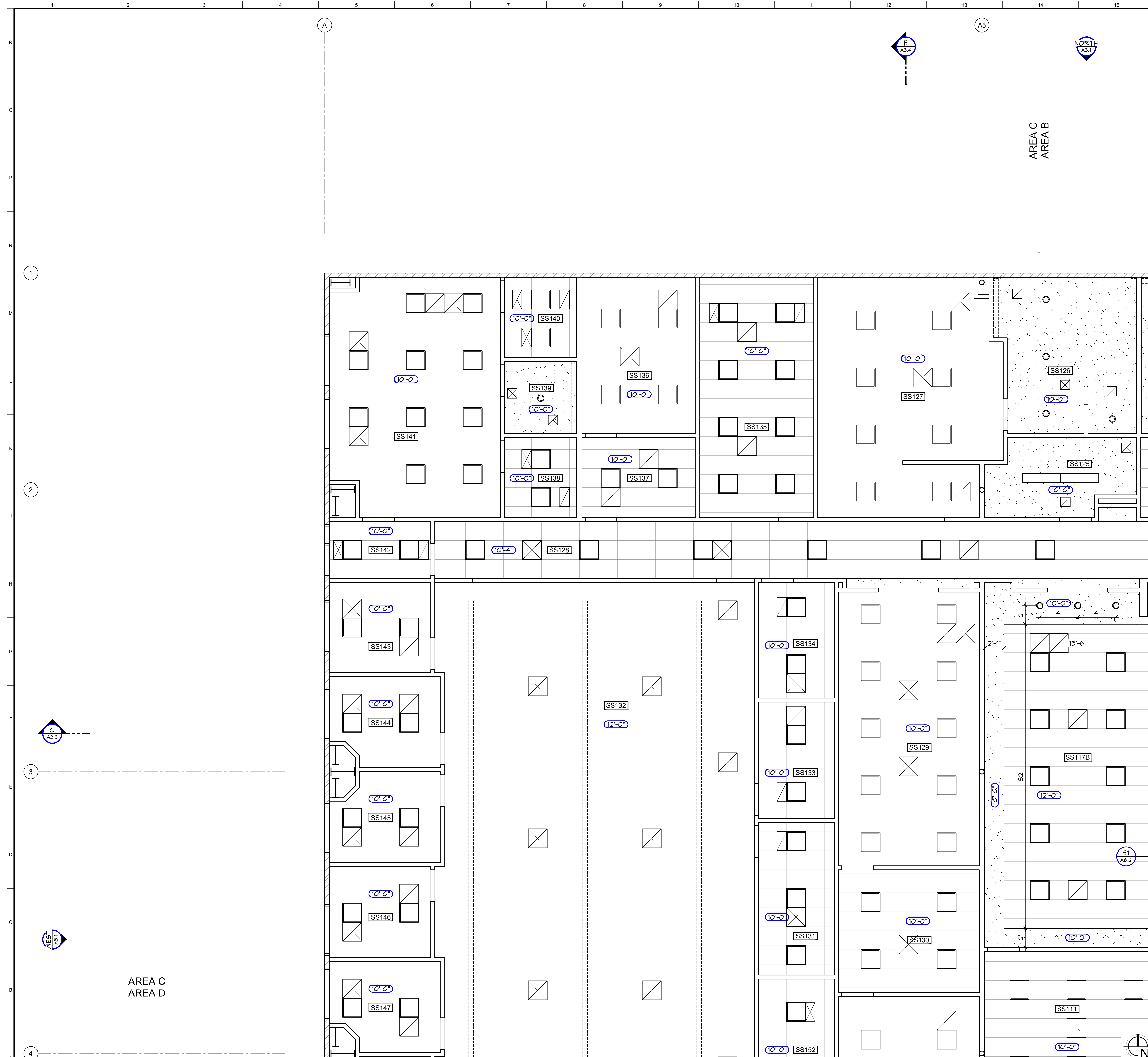
A1 REFLECTED CEILING PLAN - AREA C
