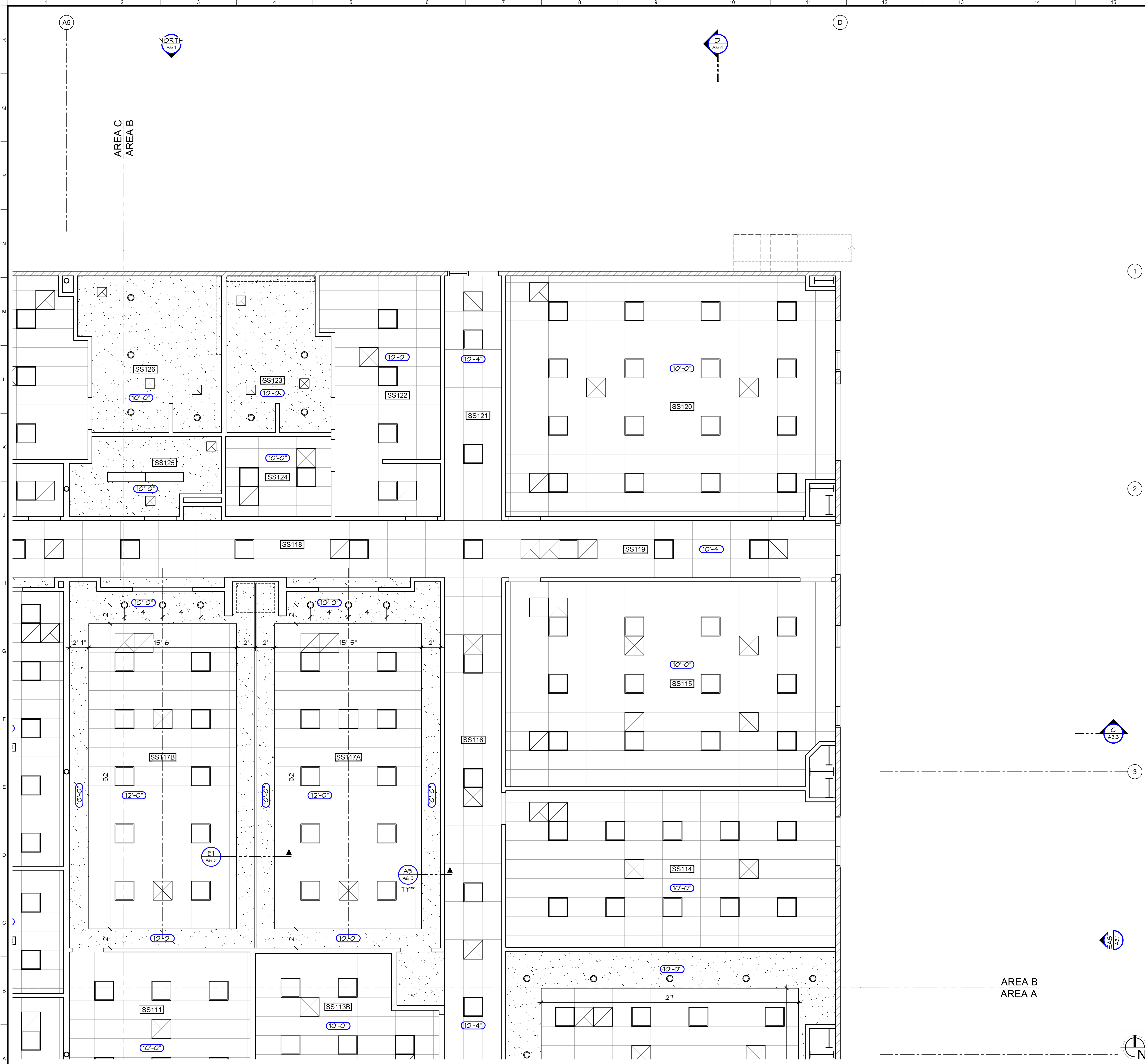
A1 REFLECTED CEILING PLAN - AREA B
