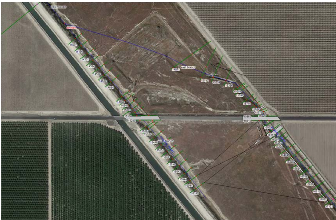
Figure 5: Plan view of HEC-RAS cross section (downstream sections based on LiDAR data not shown)
