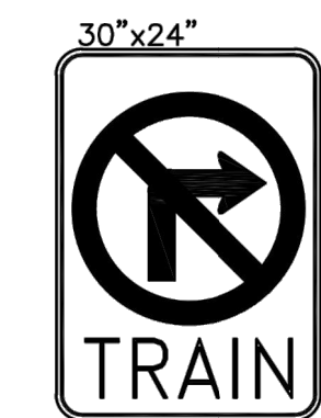
30"x24" TAPCO (R3-1) ACTIVATED LED BLANK-OUT SIGN OR APPROVED EQUAL FOR POLES I & J DETAIL "A" NTS
