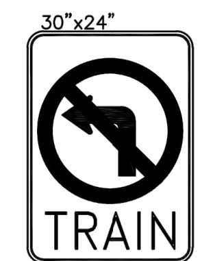
30"x24" TAPCO (R3-2) ACTIVATED LED BLANK-OUT SIGN OR APPROVED EQUAL FOR POLES A & F DETAIL "B" NTS
