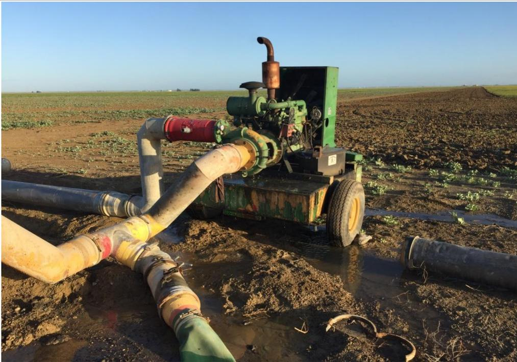
Site 1 (Figure 2): Trailer mounted diesel powered pump located at southwest corner of APN 028-071-47T.
