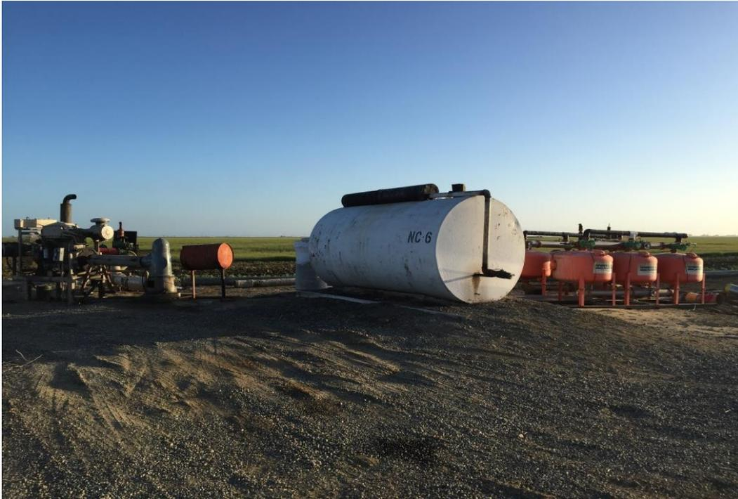
Site 1 (Figure 2): Southwest corner of APN 028-071-47T. Fuel AST, diesel powered agriculture pump, trailer mounted diesel powered pump, agriculture well, turbine oil tank and agriculture chemical filter station.
