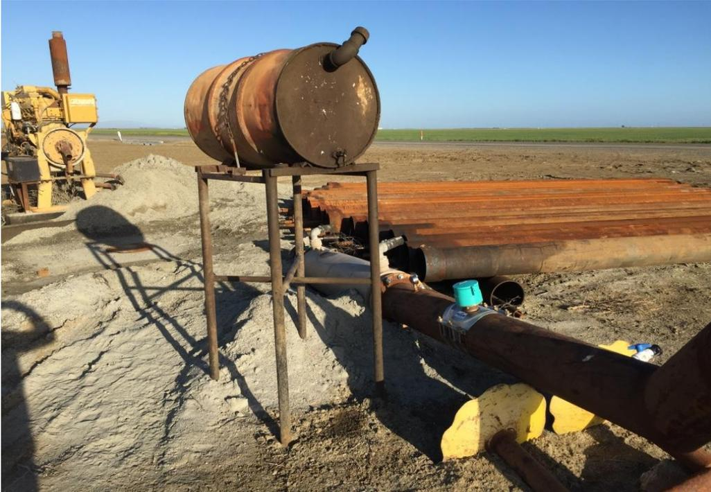
Site 2 (Figure 2): Turbine oil tank with soil staining located at northeast corner of APN 028-120-62ST.
