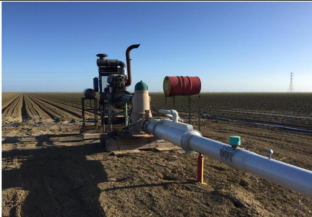
Site 3 (Figure 2): Agriculture pump, agriculture well, diesel agriculture engine, turbine oil tank and engine oil tank.
