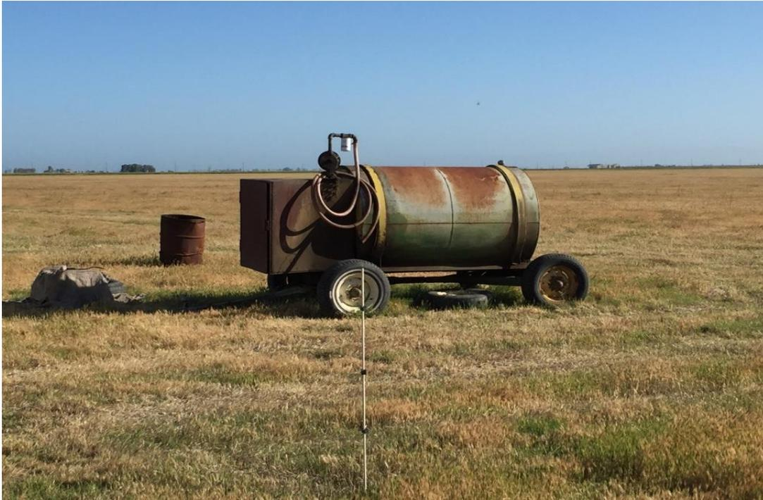
Site 5 (Figure 2): Trailer mounted fuel AST and 55 gallon drum.. No staining or stressed vegetation near tank. 55 gallon drum is empty. Located at center of APN 028-111-01ST.
