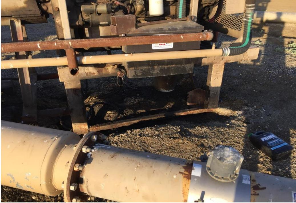
Site 1 (Figure 2): Diesel agriculture pump engine with soil stain underneath located at southwest corner of APN 028-071-47T. Empty oil container located next to engine.
