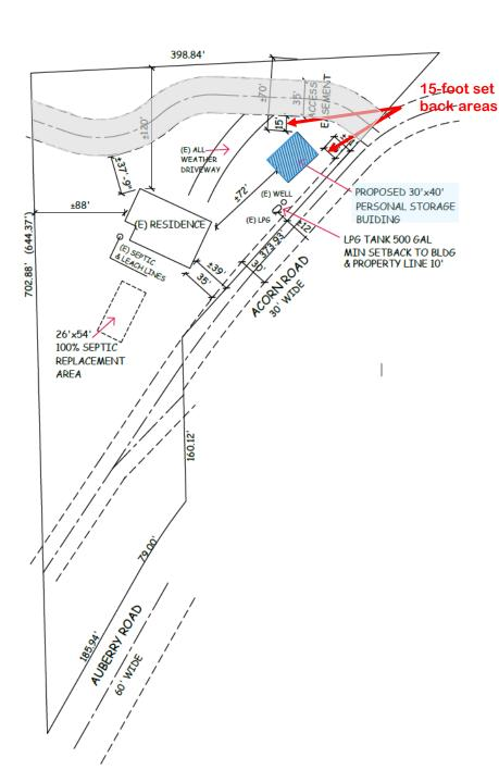
PROVIDE 2% SLOPE AWAY FROM THE PROPOSED BUILDING FOR A MIN OF 5' NO DRAINAGE ONTO ADJACENT PROPERTY DRIVEWAYS & PRIVATE ROADS SHALL HAVE A MAX SLOPE OF 12%. THE GRADE MAY BE INCREASED TO A MAX OF 20% FOR PAVED SURFACES
